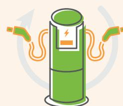
is much faster than Level 1 and 2 and can charge up to 80% of battery capacity in about 30 minutes. Charging locations tend to be close to major highways.
