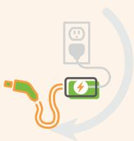
provides power using a standard 120-volt household outlet. Most plug-in hybrids and battery electric vehicles come with a level 1 charging cord.
